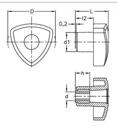
$\begin{array}{ll} d &= 50 \\ d1 &= 19 \\ d \ 6H = M10 \\ L &= 35 \\ l2 &= 19 \end{array}$
